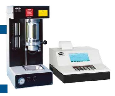
The HIAC 8011 liquid particle counting system provides immediate particle concentration data for low and high viscosity fluids. Composed of a light obscuration or dual-mode sensor, the HIAC 8011 system pressurizes fluid in a HIAC ABS-2 (Automatic Bottle Sampler) for precise volumetric sampling of industrial fluids.
